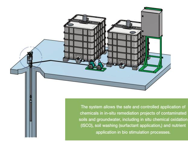
During In-Situ Chemical Oxidation (ISCO) projects, some parameters such as pressure and temperature must be controlled during the application, and safety measures also must be taken care during product handling.
