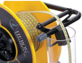
Figure 3 Hanger to support the meter at the well head. Tape Guide to protect the tape from sharp edges.
