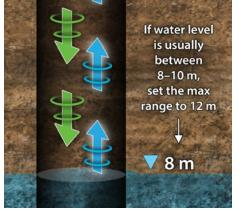
In general, knowing the approximate water level before measuring allows you to set a minimum depth to start detecting, and a maximum depth to listen for the returning pulse. For example, if depth to water is usually between 8–9 m, set your minimum to 7 m and your maximum to 10 m for higher accuracy.
