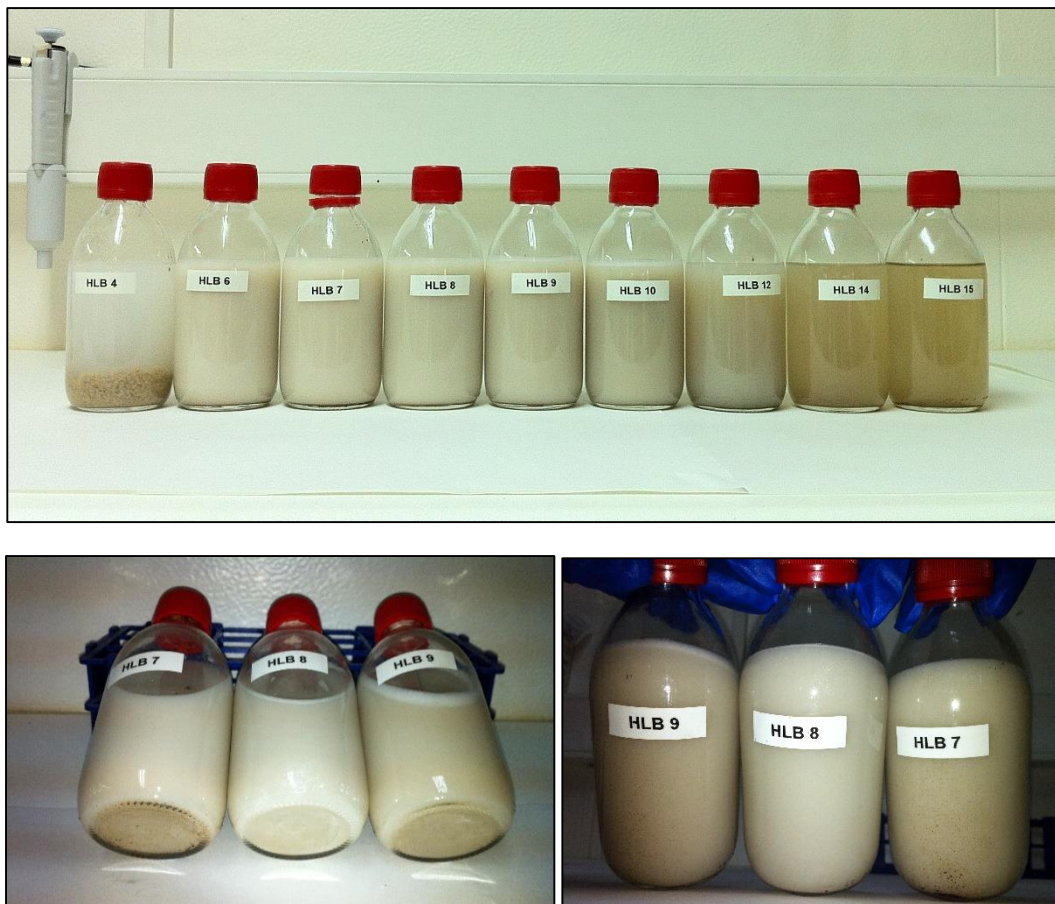
Figure 2. Determination of the required HLB for HCH DNAPL
