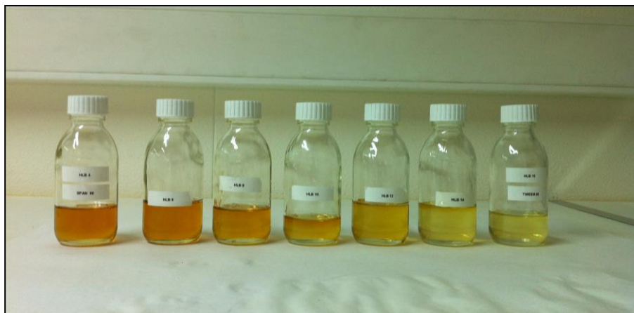
Figure 1. Series of jars of nonionic surfactant blends used in the HLB determination
