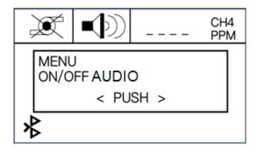
The audible alarm can be enabled or disabled by using the ON/OFF AUDIO menu option and pressing the "OK" button.
