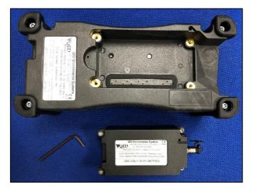
Battery pack removed from instrument
