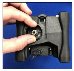
To remove the filter, rotate the filter assembly counter clockwise. The filter then unplugs from its housing.
