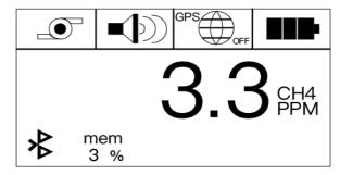
While a menu is active, the gas value is displayed in the upper right corner of the display [D].
