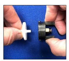
Once the filter has been replaced, re-assemble by rotating the filter assembly clockwise
