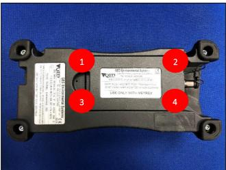
Unscrew the four battery screws
