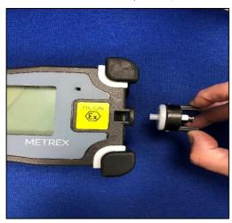
Replacement filter Part No: H-201271 Replacement filter housing Part No:H-201283-GREY
