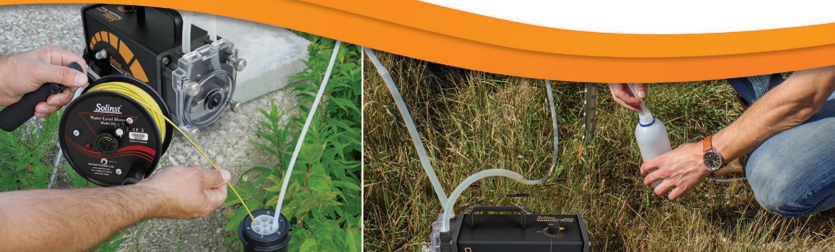
Sampling from a Solinst Model 615 Drive-Point Piezometer
