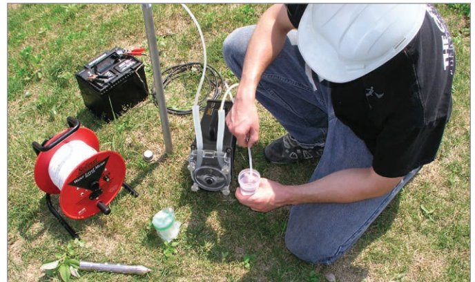
Sampling from a Solinst Model 615 Drive-Point Piezometer
