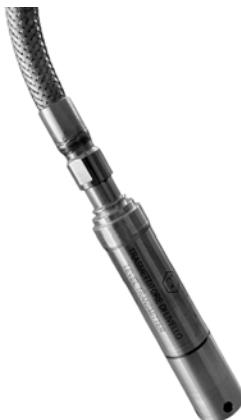
*The electronic level transmitter is a piezo resistive pressure sensor that can be used in immersion for liquid level sensing and to give analogic signal to a control system. The transmitter has been developed to work with the Officine di Trevi pumps in hard conditions, to pump wastewater, leachate and viscous liquids, hydrocarbons.*
