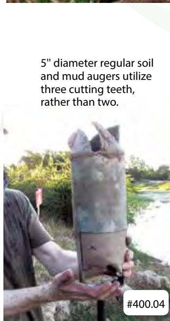
#400.06 Augers create a borehole wider than the cylinder for easy removal.
