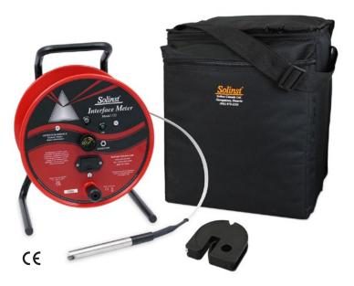
If there is only water in the well and no product, there will only be intermittent (water) signals. The presence or absence of dense (sinking) non-aqueous layers (DNAPL) is determined by continuing to lower the probe to the bottom of the well.
