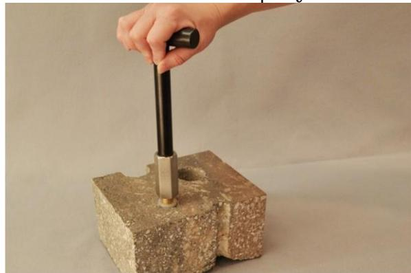
Figure 7. Removing the VAPOR PIN® sampling device
