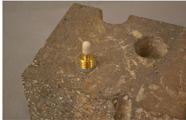
Figure 3. Installed VAPOR PIN® sampling device
