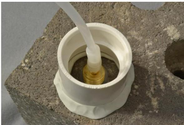
Figure 6. Water dam used for leak detection
