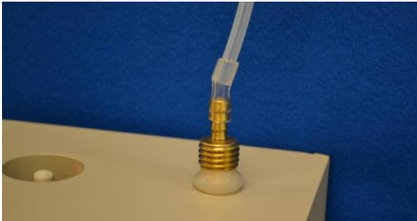
Figure 5. VAPOR PIN® sampling device sample connection
