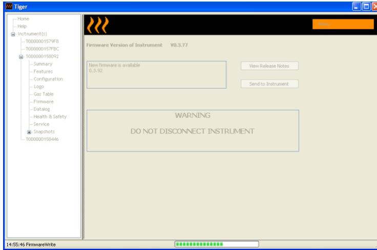
A bar at the bottom of the screen will indicate the progress of the update.
