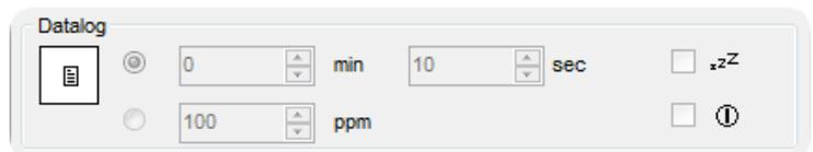
*Sleep:* When the interval between data log is >2 minutes the sleep (z-z) function becomes available. When selected, the instrument will sleep between logs therefore preserves battery life.
