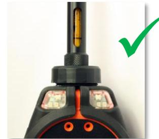
**IMPORTANT:** For best results, the pipe between the calibration cylinder and instrument should be as short as practically possible.
