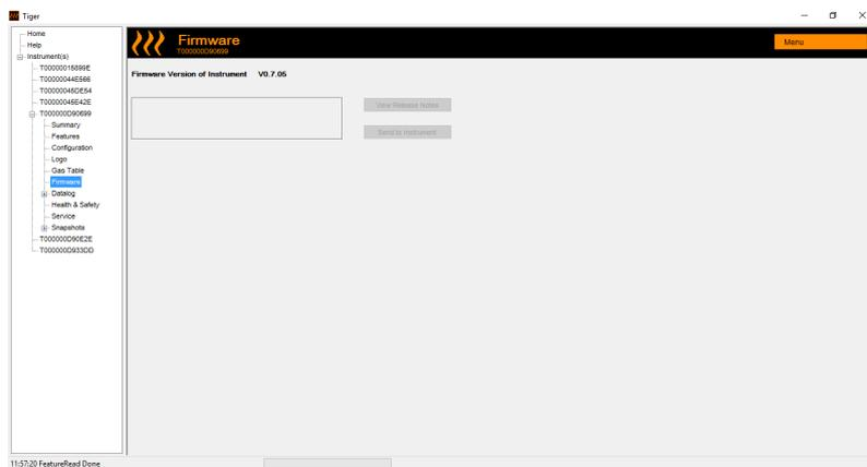
When you are ready to send the new Firmware to the instrument. Select 'Send to Instrument'.
