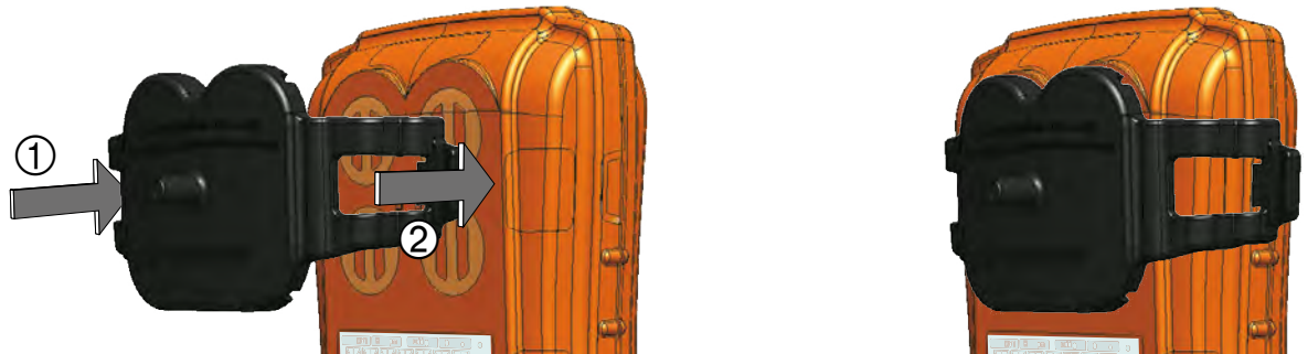
Figure 5: Fitting the calibration/bump test plate
