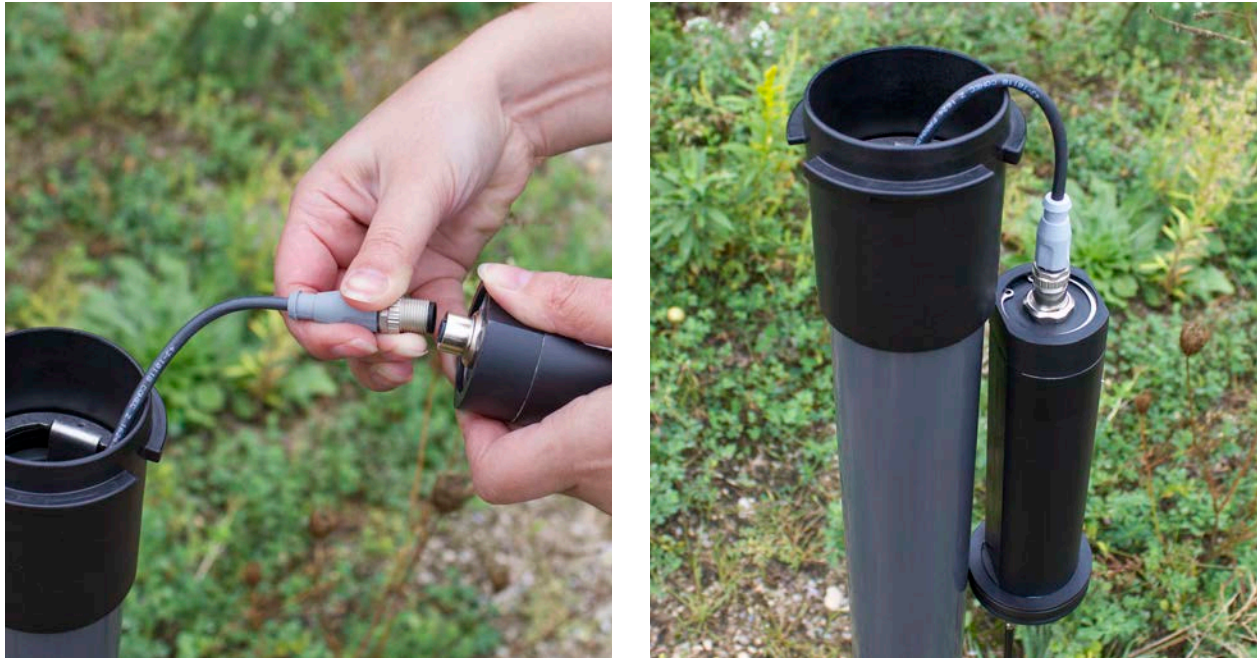
Figure 6-7 Connect the Reader Cable to the LevelSender
