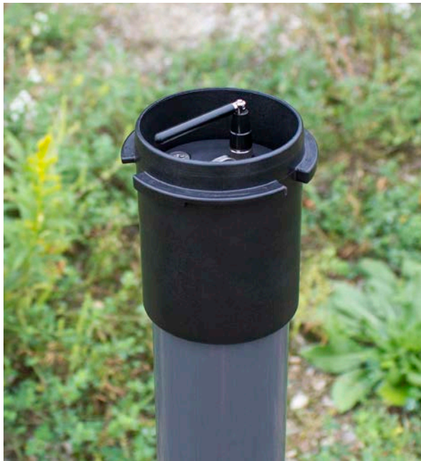
Figure 6-9 Install the Well Cap
