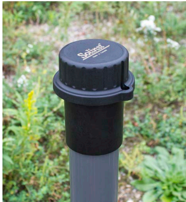
Figure 6-9 Install the Well Cap
