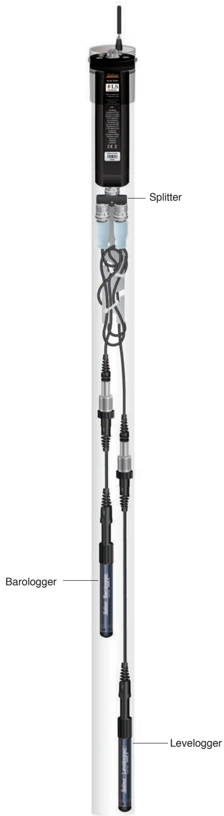
Figure 6-11 Levellogger and Barologger Installation (Reader Cable Connections Staggered)
