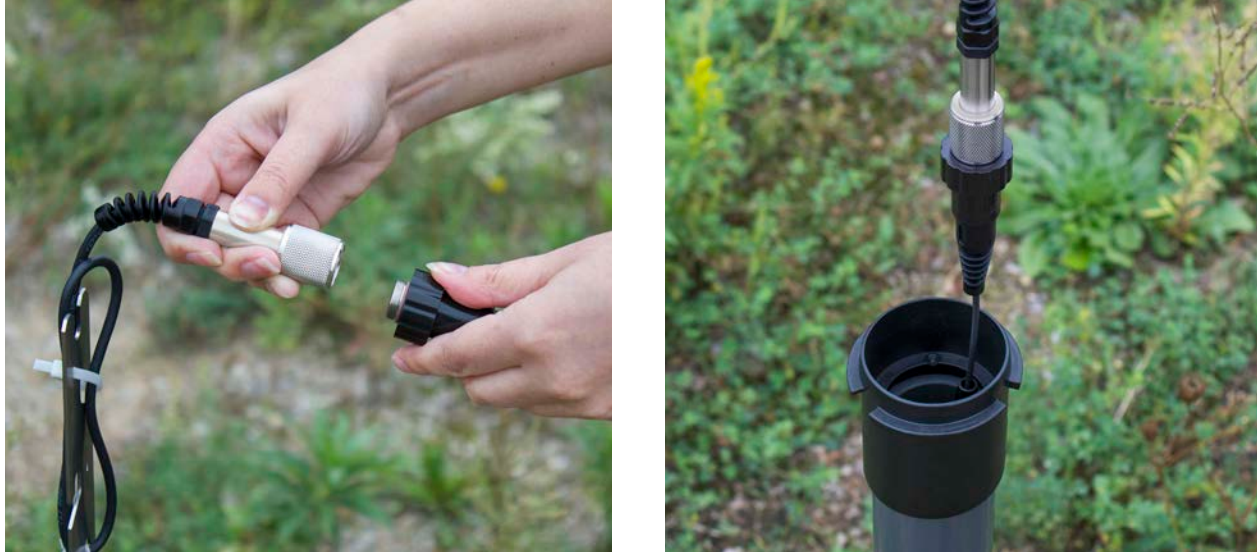
Figure 6-5 Connect the Direct Read Cable and Levelogger
