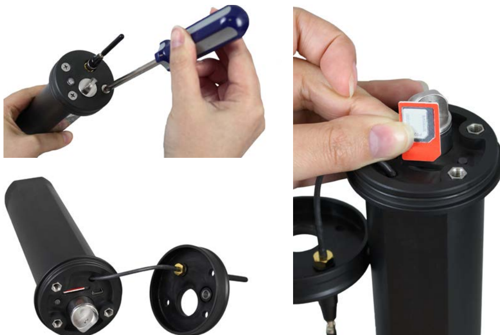
Figure 2-3 Installing the SIM Card
