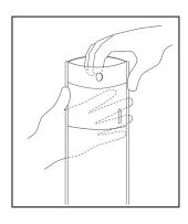
Remove HydraSleeve from package and grasp top to "pop" open. Remember to save the discharge tube for later.
