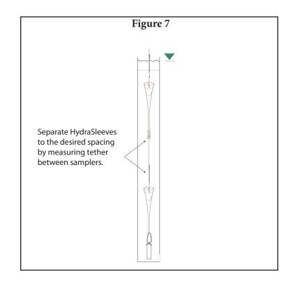
NOTE: If multiple sleeves are being used soley to provide additional sample volume, consider a single longer (often top-weighted) custom sleeve instead of multiple shorter sleeves. It's simpler and more reliable.
