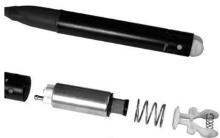
"Exploded" view of the Probe showing the pump, filter, spring and end cap
