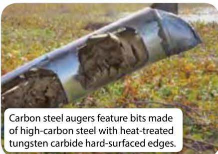
Carbon steel augers feature bits made of high-carbon steel with heat-treated tungsten carbide hard-surfaced edges.
