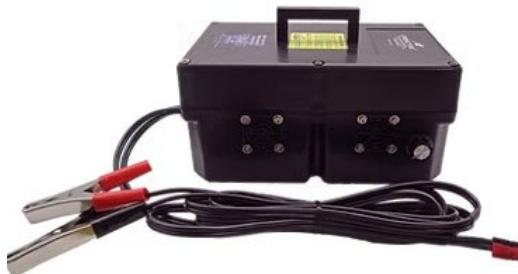
Allows to regulate the flow rate of the pumps 12 Volts. Includes protection against polarity change and thermal protection. Pump stop system. It can be regulated under flow rate up to 40ml/min. For MINI-TYPHOON, MINI MONSOON, TWISTER, TORNADO and SUPER TWISTER pumps.
