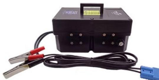
Constant voltage regulation. Allows the regulation of the flow rate of the 12 Volt pumps. Includes anti-polarity change protection and thermal protection. Pump stop system. It can be regulated under flow rate up to 40 ml/min. For MEGA-MONSOON pump.
