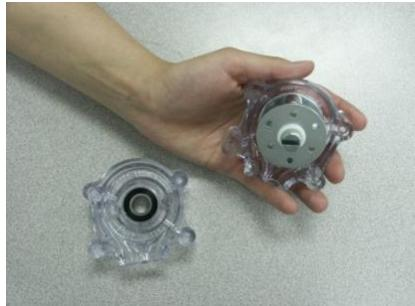
2. Place the tubing around the rollers.
